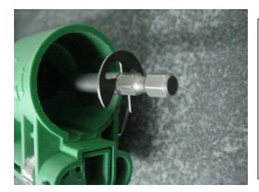
The Bit-Retaining clip is important as is prevents the hex bit from accidentally hitting the feed latch, as well as reducing problems if the bit happens to stick to a screw. Please insure that it always installed on the Hex bit before use. The adaptor assembly is only used with the Square and Phillips bits.
